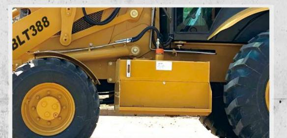
Adopt integral frame made by Q345-C high-strength steel, make the whole machine more stable, and suitable for excavating.
