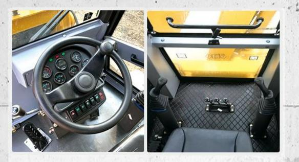
Split instrument design, more convenient maintenance; joystick operation
