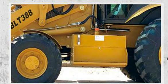
Adopt integral frame made by Q345-C high-strength steel, make the whole machine more stable, and suitable for excavating.
