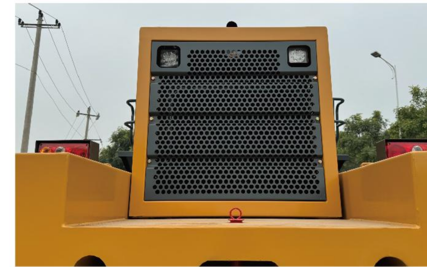
Honeycomb type heat dissipation hood, effectively improve heat dissipation performance. 蜂窝型散热器罩, 有效提高散热性能。
