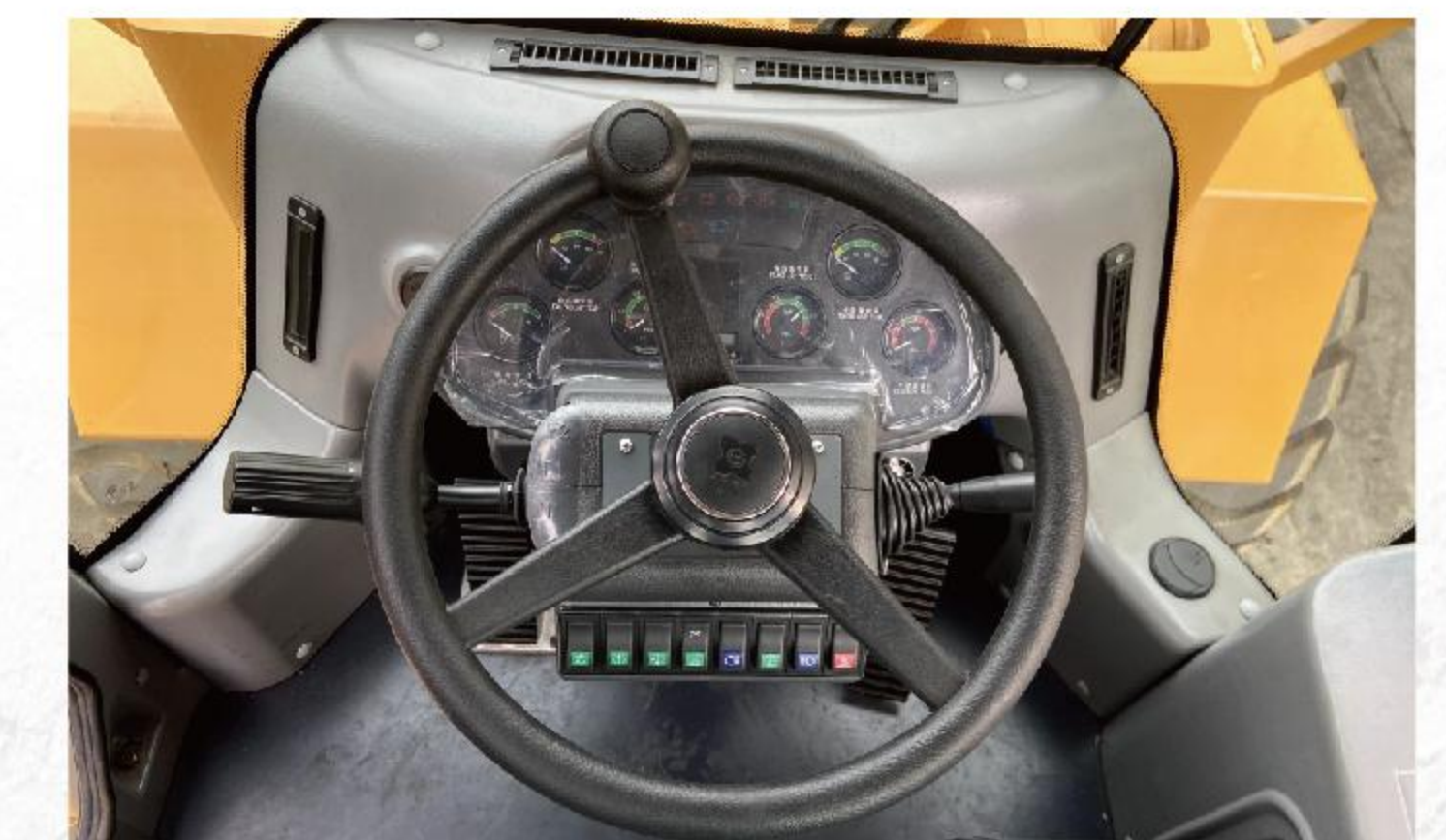
Multi-functional cab, combined instrumentation real-time display of vehicle operating status, can quickly identify fault information. 多功能驾驶室, 组合仪表实时显示车辆运行状态, 可快速识别故障信息。
