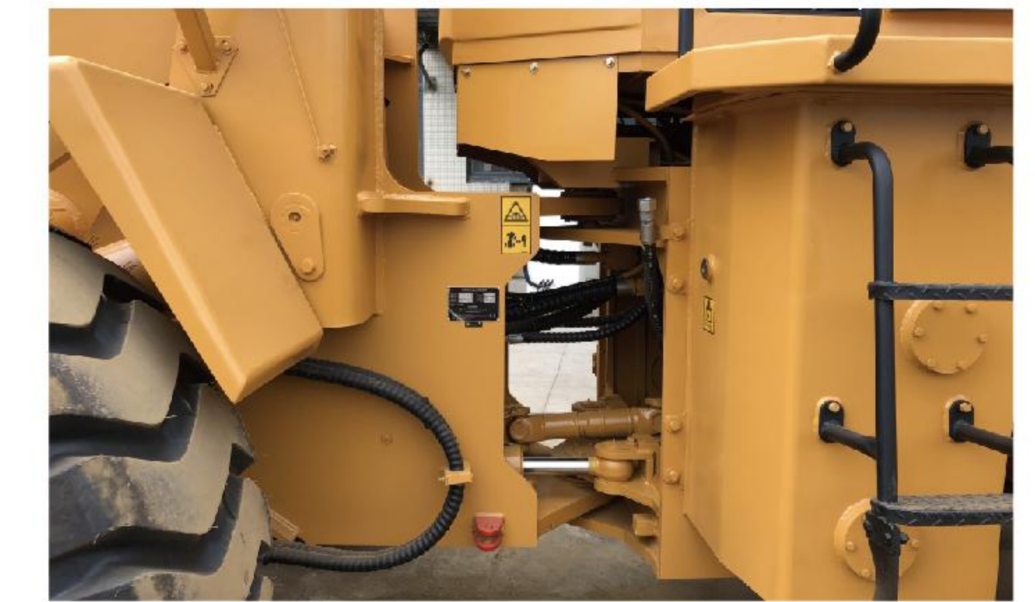
The front and rear frames have a large articulated, heavy-duty design to improve bearing life. 前后车架采用大铰接、重载型设计, 提高轴承使用寿命。
