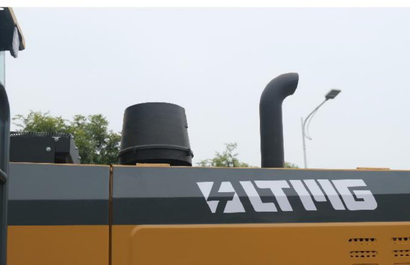
The exhaust system is equipped with an exhaust flame arrester and a spark arrester to ensure the safe operation of the whole machine in a dangerous environment.
