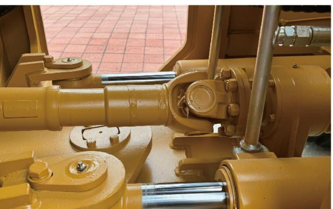
The articulation adopts double tapered roller bearings, high bearing capacity, small turning radius, and swifter and more efficient loading and unloading.
