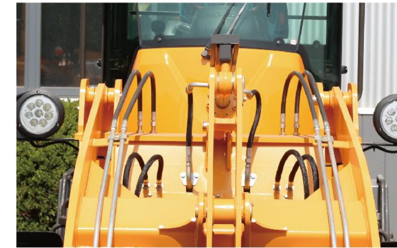
Enhanced hydraulic cylinders for robust operation and powerful lifting effect.
