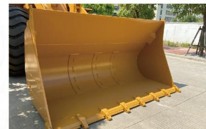
Optimise the bucket discharge plate structure, easy to discharge and reduce the impact; the service life is greatly extended.
