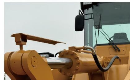
Adopting large-displacement double-pump merging hydraulic system, with large cylinder power, fast arm lifting and faster loading speed.
